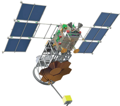
Fig. 2: Detector TUS on-board Lomonosov satellite
